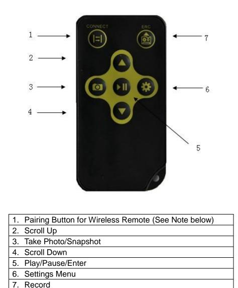
**Note:** When attempting to use the remote control for first time, it may need to be paired to the DVR first. Please enter the DVR menu to set the device into pair mode. Then select the Connect button on the remote to pair it with the DVR.
